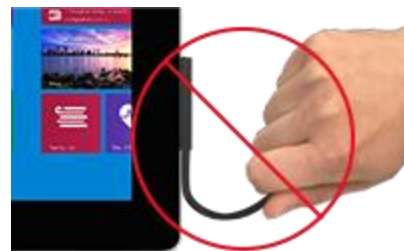
Incorrect: Tugging on cord to unplug
